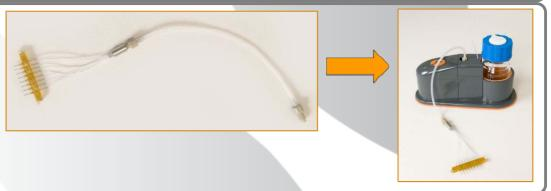
**4.** Connect biochip outlet cable as shown.
